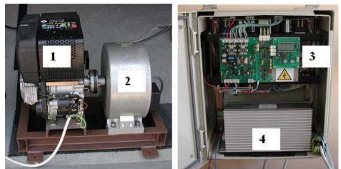
Figure 2. The EGS experimental model (1: diesel engine; 2: SGPM; 3: ac-dc converter; 4: filter)
