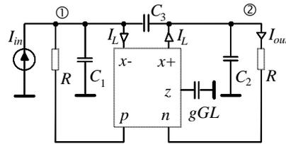
Figure 8: Economical simulation of the ladder filter in Fig. 6 with symmetrical termination.
