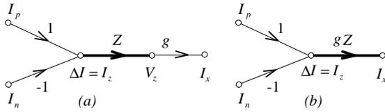
Figure 3: (a) „IVI“ flow graph of CDTA element with grounded load across the  $z$  terminal, (b) simplified flow graph after skipping the voltage node.
