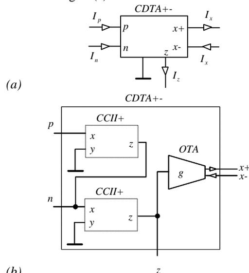
Figure 2: (a) Symbol of the CDTA element, (b) its implementation by current conveyors and by OTA with double current output.
