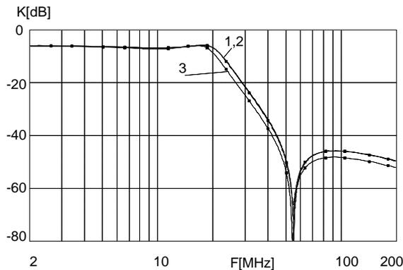
Figure 10: Frequency response of ladder filter in Fig. 6 (1) and the simulated responses of CDTA-based leapfrog structures in Fig. 7 (b) (2) and Fig.8 (3).
