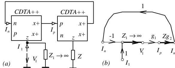
Figure 9: (a) impedance inverter with two CDTAs, (b) the corresponding „IVI“ graph.
