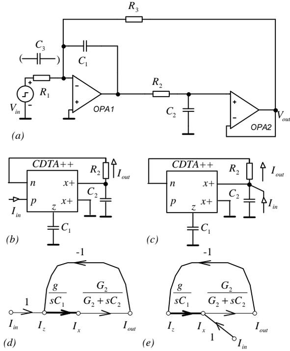
Figure 5: (a) LP (with  $R_1$ ) or BP (with  $C_3$ ) biquad, (b) CDTA-based LP filter, (c) CDTA-based BP filter, (d), (e) the corresponding reduced „IVI“ graphs.
