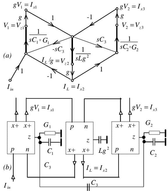
Figure 7: (a) „IVI“ filter flow graph, accordant with equations (2), (b) the synthesized filter.
