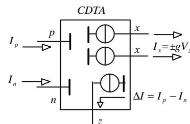
Figure 1: Behavioral model of CDTA element.
