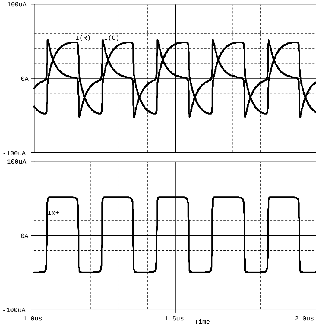
Fig. 5: Waveforms of circuit in Fig. 4. R = 1.5k\Omega , C = 10pF . Repeating frequency is 5.2MHz.
